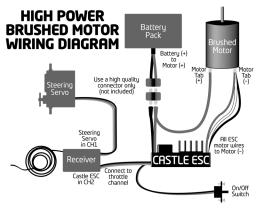
connect to the red wire (or positive + side hood) on your motor, and the black wire to the black wire (or negative - side hood) of the motor. The white motor wire (or center connector on the ESC) is not used. After calibration, (explained later) you may need to swap the two motor wires to get the wheels to spin in the right direction.
